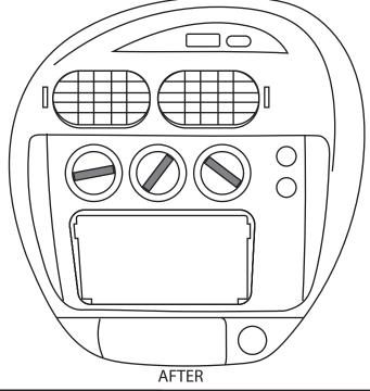
6 Connect all cables and harnesses and push full assembly into the dash, ensuring all clips have locked into place.
