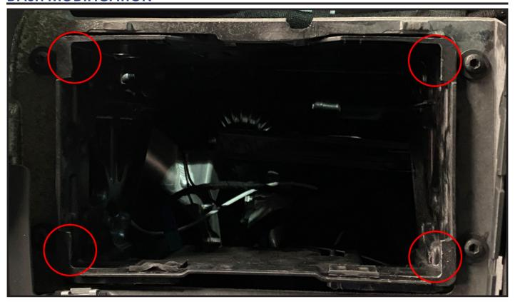
At this point you will need to modify the dashboard. Using a file or a cutting tool, begin to file away the inside lip of the four highlighted corners of the main dash cavity.
