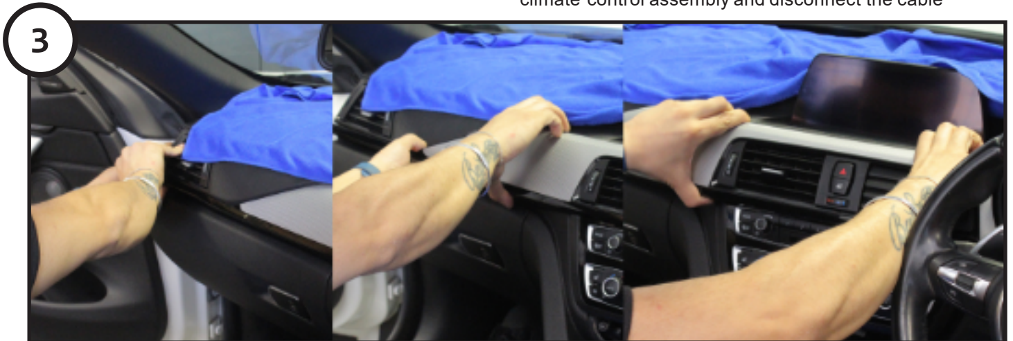
3 Use a panel removal tool to partially remove the air vent panel/vents, starting from the left hand side of the dashboard and moving to the centre
