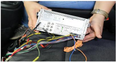
8. Connect the USB adapter to the back of the Radio (this goes to the factory dashboard USB connection)
